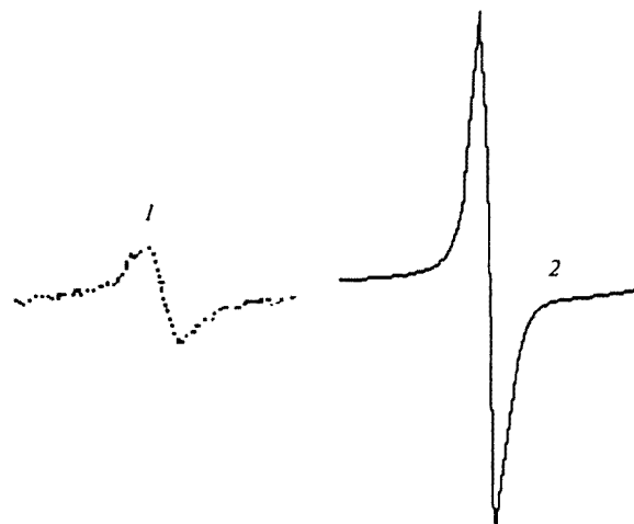
Fig. 2. ESR spectra: 1, polyaniline film in the base form; 2, polyaniline film doped in a solution (1 M ) of \text{ZnCl}_2 at pH 5.5.
